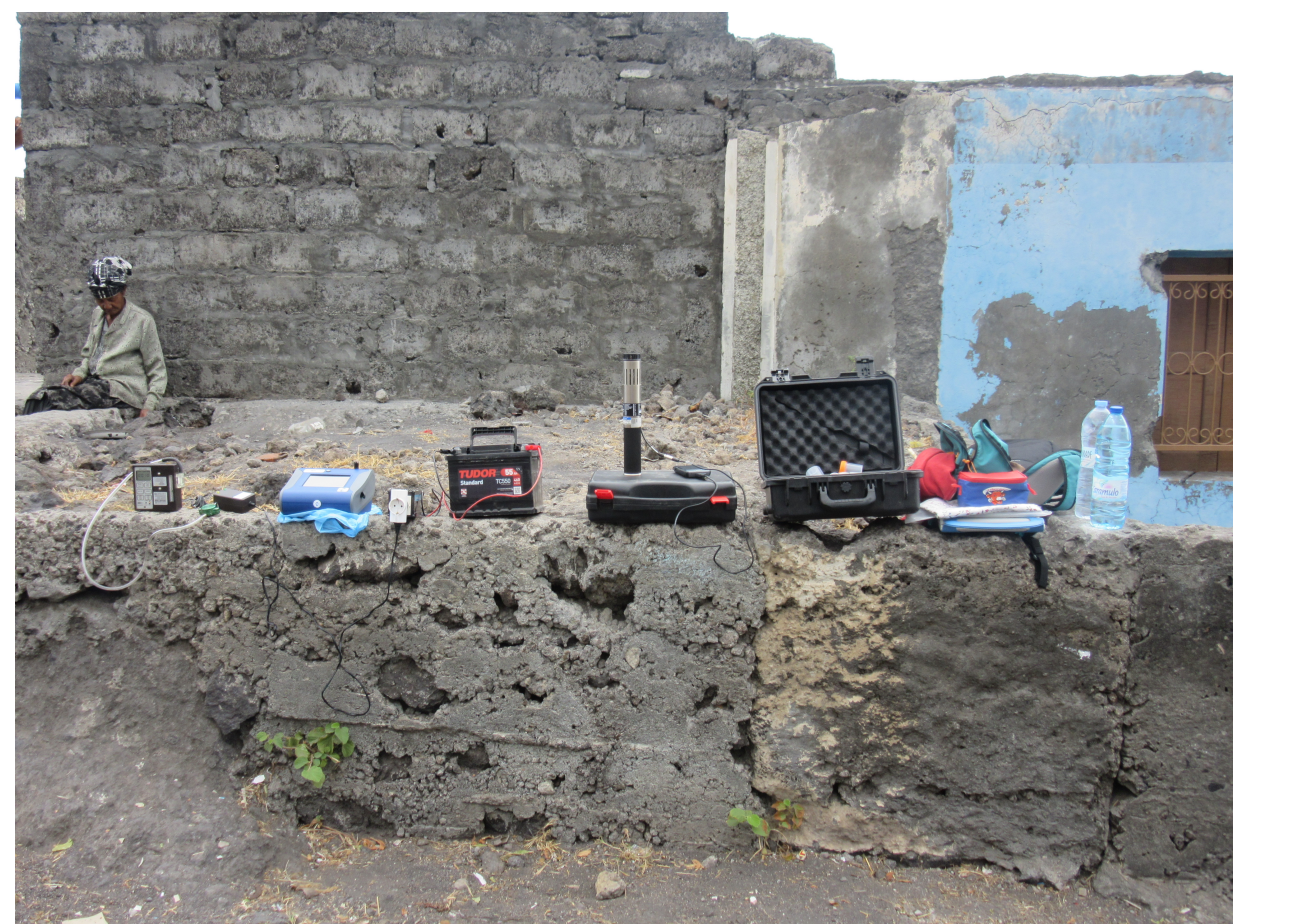
Fig. 5 - Air quality monitoring portable equipment: (a)PM10 sampler, (b) dust track aerosol monitor, and (c) CO, CO2, TVOCs, temperature and humidity analyzer.
